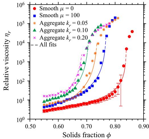
Figure 2. Divergence of the relative viscosity  $\eta_r$  with area fraction  $\phi$  at  $\dot{\gamma}^* = \infty$  for each of the suspension types explored. Shown in dashed lines are fits to  $\eta_r = \nu(1 - \phi/\phi_m)^{-\lambda}$ . The maximum solid fractions for smooth particles  $\mu = (0, 100)$  and aggregates with  $k_r = (0.05, 0.10, 0.20)$  are, respectively,  $\phi_m = (0.84, 0.77, 0.74, 0.71, 0.69)$  (see table 1).
