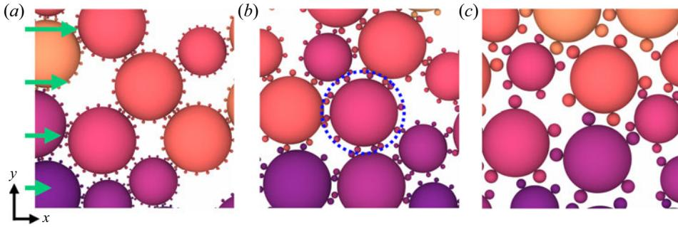
Figure 1. Schematic of aggregate particles (coloured by particle). Shown are suspensions with asperity sizes  $k_r = (a) 0.05; (b) 0.10; (c) 0.20$ . Green arrows indicate the imposed velocity profile  $u_x(y) = \dot{\gamma}y$ . Blue dashed circle represents contact with  $P = 0$  (see (3.1)).
